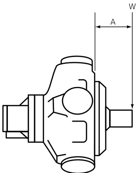
**A** = Distance from mounting face to load centre (mm)
