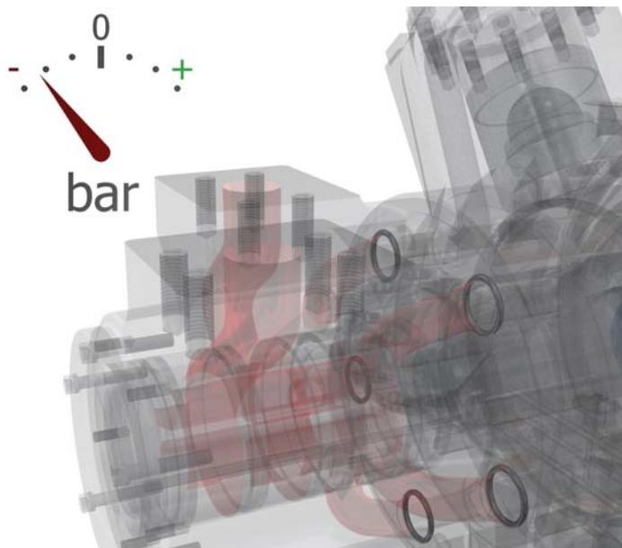
Cavitation can occur due to many different factors. Although it is not possible to make the HMC motor resistant to cavitation, certain features can be added to improve the motor's resistance to short periods of lost port pressure.
